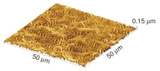
**Figure 2.** AFM picture of a self-assembled uracil-G1-PAMAM/MAP structured film
