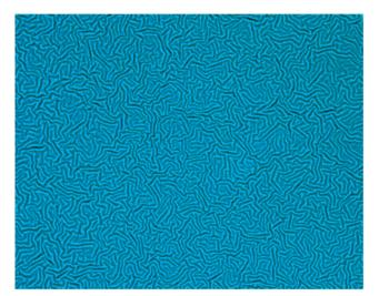
**Figure 3.** Optical microscope picture of a large area  $(1.7 \times 1.5 \text{ mm})$  self-assembled uracil-G1-PAMAM/MAP system.
