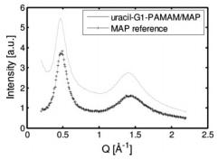
Figure 4. Wide-angle X-ray scattering data, I(Q), vs scattering momentum Q as obtained on (i) a film of self-assembled uracil-G1-PAMAM/MAP composite and (ii) on the pure MAP the matrix component.
